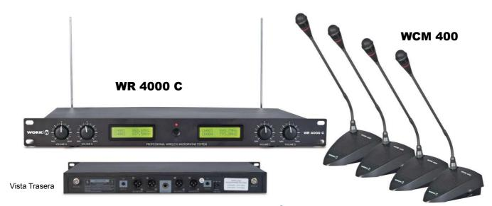
**WR 4000** is a 4 channels wireless conference system for the UHF band. This system saves the need to wire the desktop microphones, placing the receiver next to the mixing and amplification system and creating a discrete and functional system. The receiver incorporates two LCD screens, each of which show the frequency information and status of two channels. Each channel has independent volume control located on the front panel.
